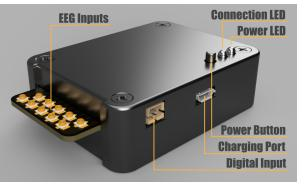
**Charging port.** The device's battery can be charged via micro-USB port using standard 5V chargers such as mobile phone chargers with micro-USB plug. The charger should be capable of providing at least 800 mA of current. Do not use the device when charging with chargers powered from grid electricity due to safety reasons and potentially 50/60 Hz noise affecting the signals. The device can be used when charging from power bank though.
