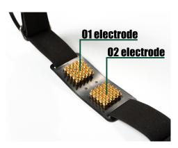
**Fp1 and Fp2 electrodes.** There are two frontal electrodes with golden pads as well, placed approximately at Fp1 and Fp2 locations.
