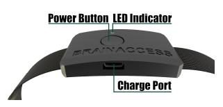
**LED indicator.** The breathing blue light indicates that the device is turned on. If a Bluetooth connection is established between a computer and the device it turns solid blue. When the battery level drops below 15% the red light fast-blinks a couple of times on each 1% drop. When the device is charging, the red light is fading-in. Once fully charged the red light turns off.
